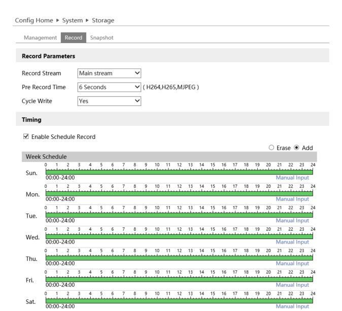
Click the desired record event such as motion, intrusion, tripwire, face detection. You will need to enable the function. Reference the individual document for motion or analytic function configuration. **Motion will be used in the example.**
